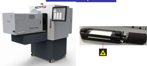
Figure 1: Left: A commercially available integrated SPECT-PET-Optical-CT (MILabs B.V., Utrecht, The Netherlands) was upgraded with a continuous wave near-infrared laser diode (730 nm). Right: A partially transparent mouse holder with integrated anesthesia and heating system, built-in marker holes for robust fusion, compatible with SPECT and PET, was designed and produced using 3D-printing.
